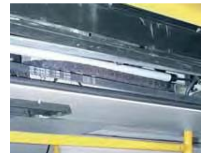
Sliding door in subway with igus® chainflex® CF9 cable for smallest spaces
