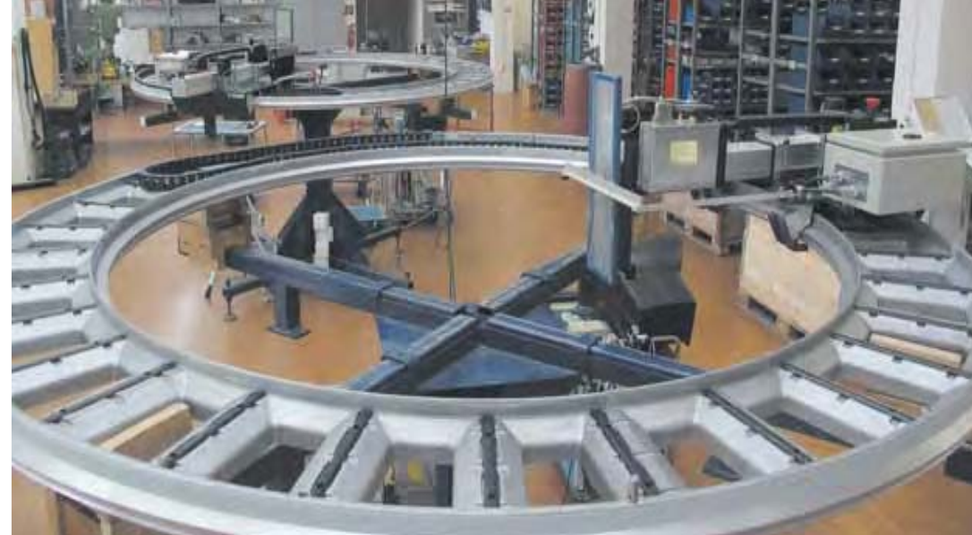
E2 mini e-chain®, RBR-version with reverse bending radius
