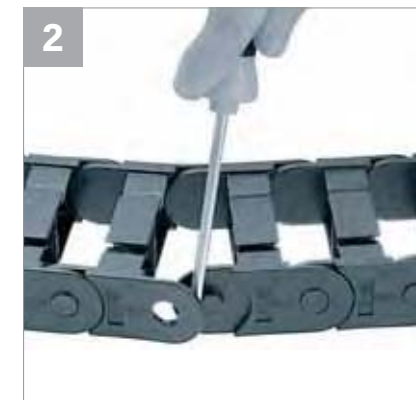
Release side link, twist and pull apart
